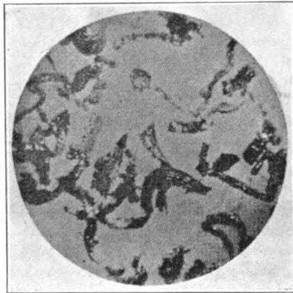
Photomicrograph of chips from a grinding wheel
